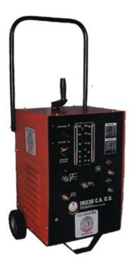
**APPLICATION**: When used with DC, IW-235 CACD provides a mild, stable arc. Its AMP range covers from 40 to 160 Amperes. This is enough for AC welding rods up to 5/32" (4.0 mm) in diameter. With AC you can use conventional type welding rods like: E 6013, E 6011, E 7018 CA and special AC welding rods (stainless steel and cast iron).
